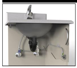
This illustration shows a typical installation for the Model 1720 Tapmaster. The valve blocks are connected in-line on the hot and cold water supplies with 3/8" O.D. compression fittings. The pilot/actuator valve is mounted about knee height on the inside wall of the cabinet opposite the door hinge. The control tubing is routed in between the valves. Water flow to the faucet is activated by pressing with the knee or leg against the cabinet door.
