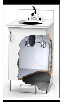
This illustration shows a typical installation for the Model 1750 Tapmaster. The valve blocks are connected in-line on the hot and cold water supplies with 3/8'' compression fittings and the kick plate is mounted on the cabinet toe kick with the control tubing routed in between them.
