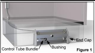
Start by determining whether the control tubing will be routed through the base of the kick plate as in **Figure 1**, or through the kick plate end cap as in **Figure 2**. It is recommended the kick plate be positioned as to be aligned with the center of the faucet/ sink. Alternately, it may be positioned to best suit the needs of the end user.
