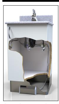
This illustration shows a typical installation for the Model 1751 Tapmaster. The valve blocks are connected in-line on the hot and cold water supplies with 3/8" O.D. compression fittings. The pilot/actuator valve is mounted about knee height on the inside wall of the cabinet opposite the door hinge. The kick plate is mounted on the cabinet toe kick. The control tubing is routed through the cabinet base to the hot and cold water supplies to make the connections to the valve blocks.
