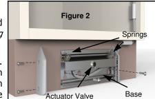
**STEP #4** - Remove the end cap. Slide the cover back on the kick plate base, by pressing down on each spring in succession while the cover is slid on. Remount the end cap.
