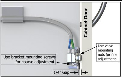
First determine a height location where the pilot/actuator valve is to be mounted on the inside of the cabinet opposite the door hinge, preferably about knee height or higher. The objective is to mount the pilot/actuator valve so that the inside face of the cabinet rests against the button of the pilot/actuator valve. This will set the door ajar very slightly, about 1/32".
