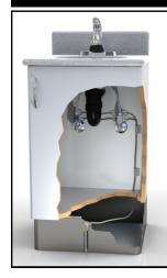
This illustration shows a typical installation for the Euro Model 1770 series Tapmaster. The valve blocks are connected in-line on the hot and cold water supplies with 3/8" compression fittings. The Euro foot activator is mounted on the cabinet toe kick with the control tubing routed from the foot activator through the cabinet base to the hot and cold water supplies to make the connections to the valve blocks.
