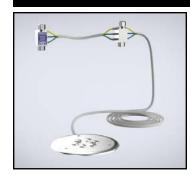
This illustration shows a typical Model 1780 Tapmaster. The valve blocks connect in-line on the hot and cold water supplies with 3/8" O. D. compression fittings. The pilot/actuator valve is mounted to the underside of the activator disk which is mounted to the floor with the three #8 countersunk screws provided.
